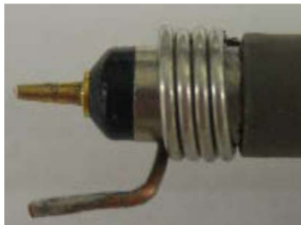
Figure 2: Wrapping bare wire to form a ground
