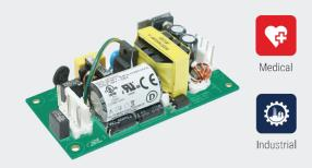
Advanced Energy's SL Power GB10 series of open-frame AC-DC power supplies comprises six single output models. All models feature medical safety approvals and accept a universal input of 90 to 264 VAC. These compact switch-mode power supplies feature output overvoltage, overload protection, with short-circuit protection on the output. GB10 series power supplies provide 12 Watts of output power with free air convection cooling.
